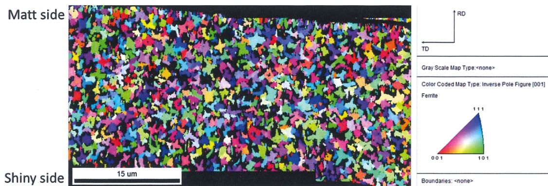
Figure 1. EBSD analysis of cross-section of annealed FeSiBC amorphous ribbon. The sample was heat treated at 450°C for 60 min.
