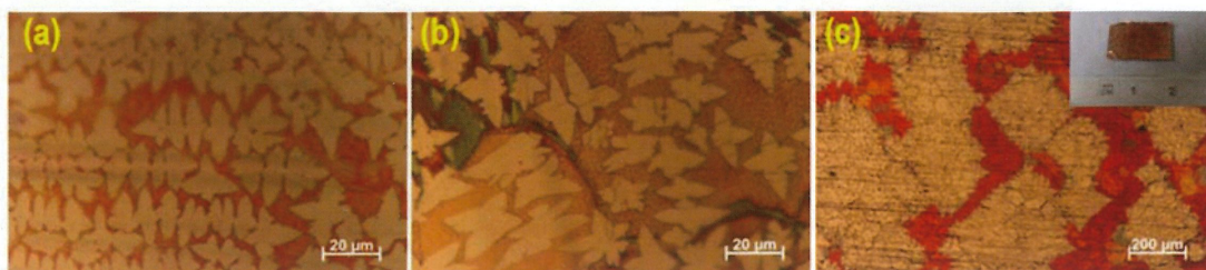
Figure 1. (a-b) Optical images of graphene grown in 20 mtorr CH 4 at 1030°C with and without electropolishing treatment of the Cu substrates, respectively. (c) Optical image of graphene grown by the O 2 -assisted CVD process.
