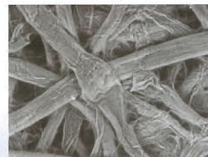
Low-vacuum mode Backscattered electron image, Original mag: \times 540 , Specimen: filter paper
