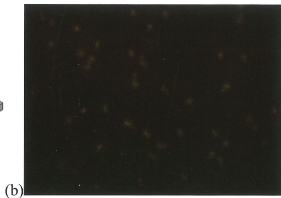
Fig 3. (a) testing stage for fluorescence light microscope (b) 100x fluorescence light microscope image for 400 nm polystyrene
