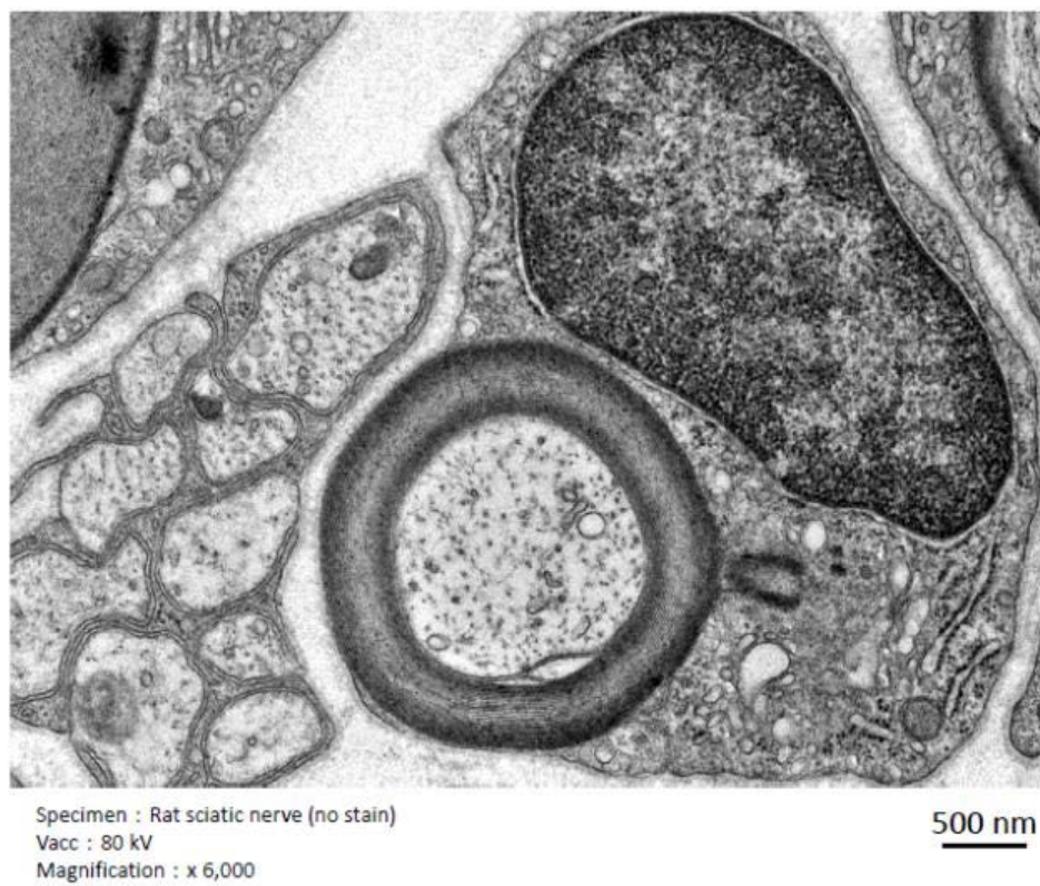
Fig. 2 TEM image by 8M-pix camera (high contrast image is obtained without staining specimen by using high-contrast(HC) mode)
