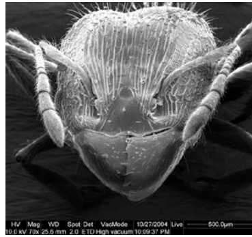
Figure 1. Viewing an ant with gold coating only with high vacuum mode.
