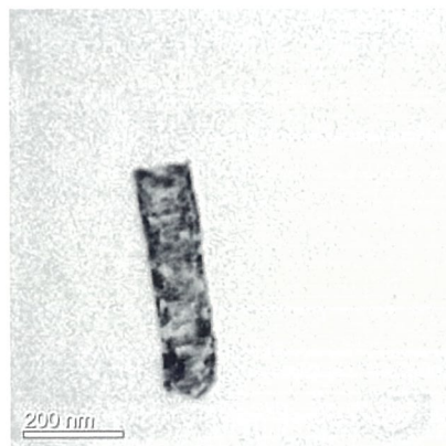
Fig.3: TEM bright-field images of the Zn-ZnO core-shell nanowire during in- situ heating and cooling when temperature is (a) at 400 °C, showing the tip collapse; (b) at 450 °C, showing only a ZnO tube left behind from Zn evaporation; and (c) cooled back to room temperature, showing the Zn nanoparticle formed on the ZnO core surface.
