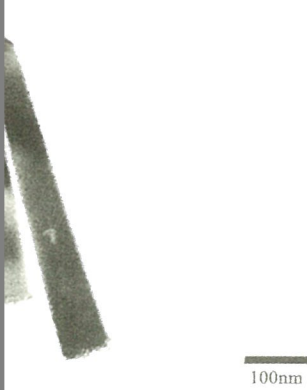
TEM image of \text{In}_2\text{O}_3 nanorods. (b) Selection diffraction pattern of (a).
