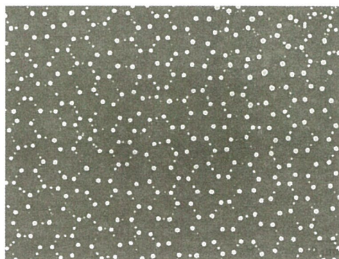
Fig. 2 SEM image of Au nanoparticles deposited sample annealed at 1000 °C for 60 min.
