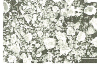
Fig. 2. SEM micrograph of powders milled for 4 h.
