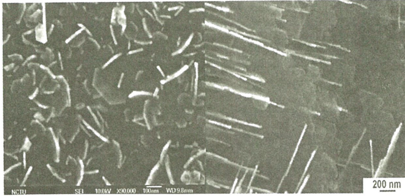
Fig. 1 SEM micrograph showing that the diamond platelet shape can be in hexagon and triangle.
