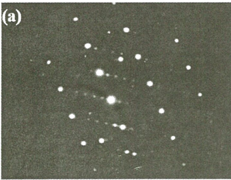
Fig. 2 Diffraction pattern of (a) \alpha_1 / \theta_1 / \theta_2 and (b) \alpha_1 / \alpha_2
