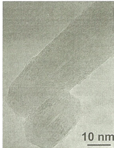
Fig.2 TEM image of the nanotube with defect free structure by the nanotube and the capsule
