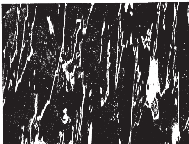
Fig. 2-Dark field image of HSLA steel, quenched from 1100°C showing retained austenite and carbides.
